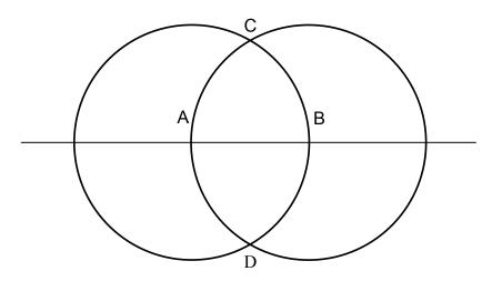
Taking the portion of our original baseline between the two centers we immediately recognize that it is a common radius to both circles, as AB below. Drawing two additional lines from the centers A and B to the end point C creates an equilateral triangle, since both lines AC and BC are radii of equal circles they must be equal to each other, that is, since both AC and BC are equal to AB, they are equal to each other, and the triangle ABC is equilateral.
